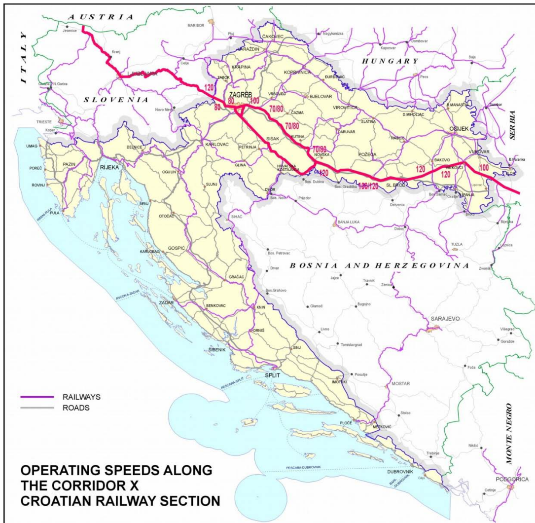
Picture 4 – Operating speeds along the Corridor X
